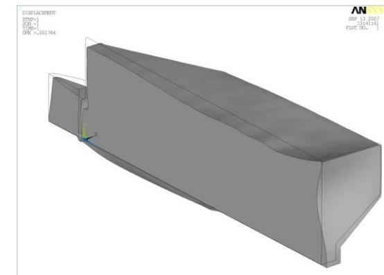
**Deformation, atmospheric pressure, RF-Power**
