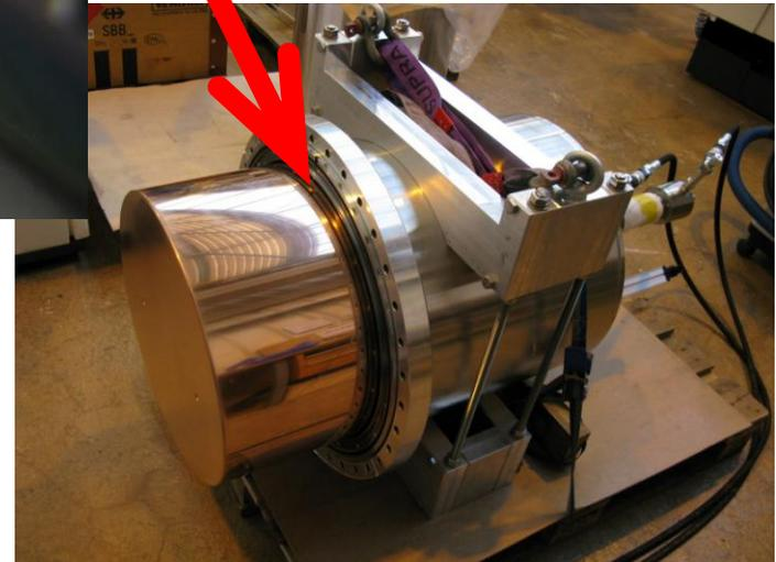
After successful high power tests, it was discovered that several RF contacts were bent.
