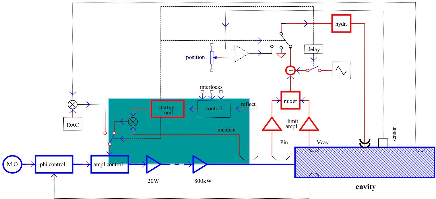
*Block diagram of the pulsing startup and interlock control circuitry*
