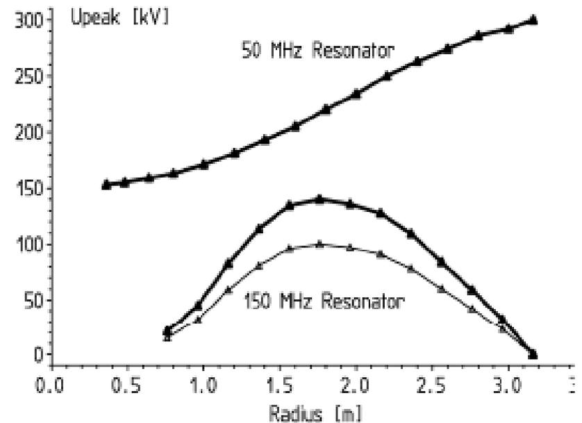
Gap voltage versus Radius of existing resonators
