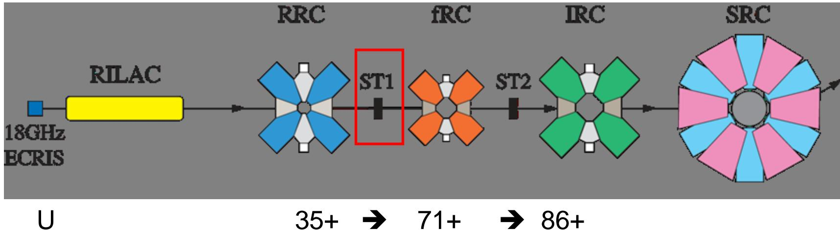
Carbon Foil  $300 \mu\text{g}/\text{cm}^2 \Rightarrow$  Lifetime < 12 hours
