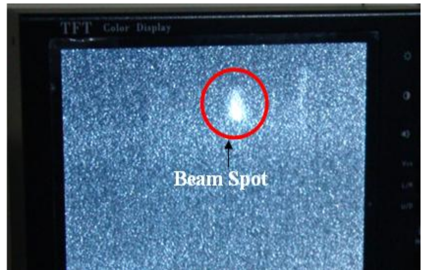
Accelerated Ne3+ Beam on viewer probe
