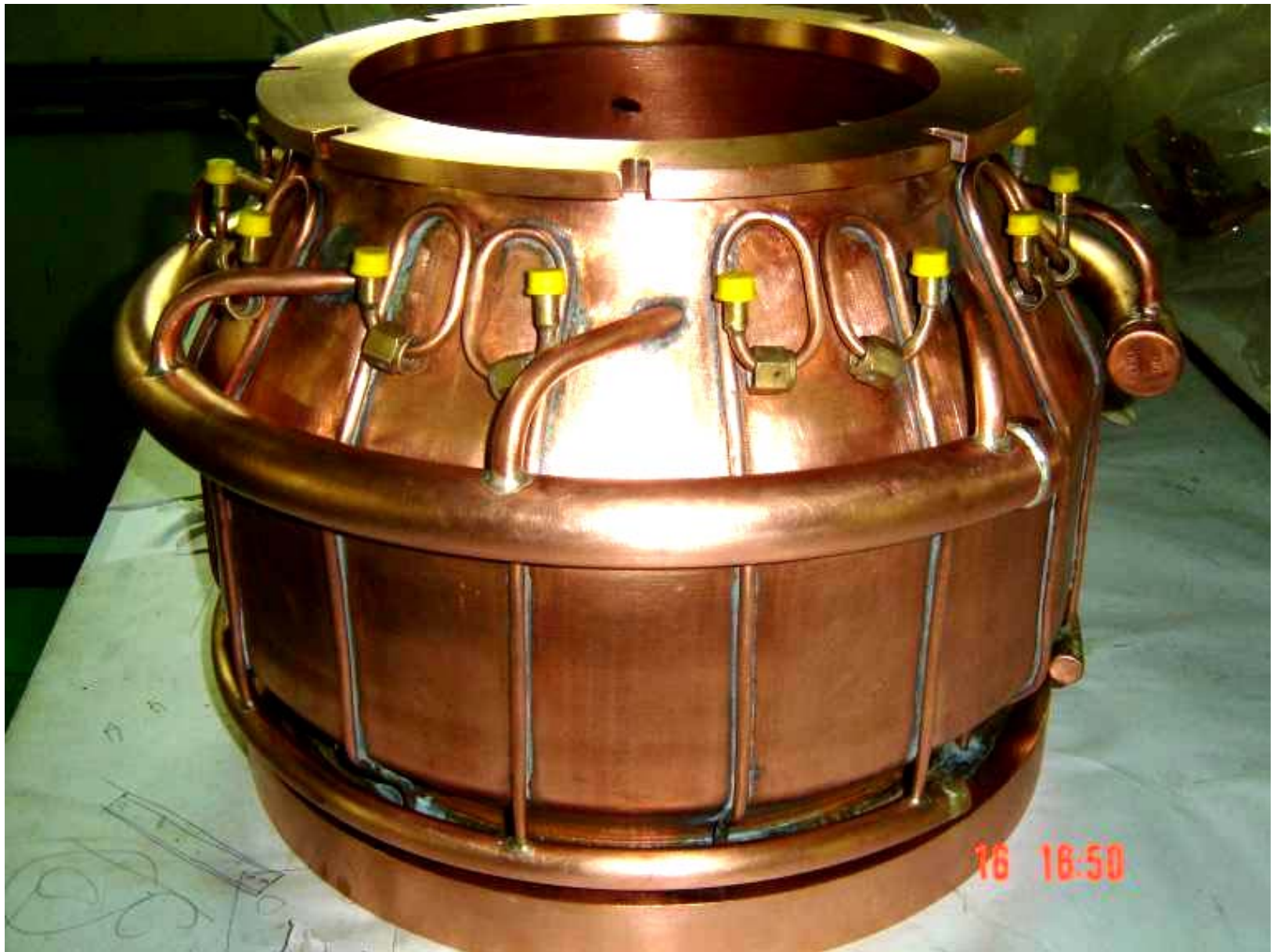
Outer Conductor Spinning
