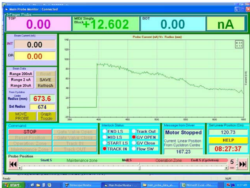
Beam current profile along radius
