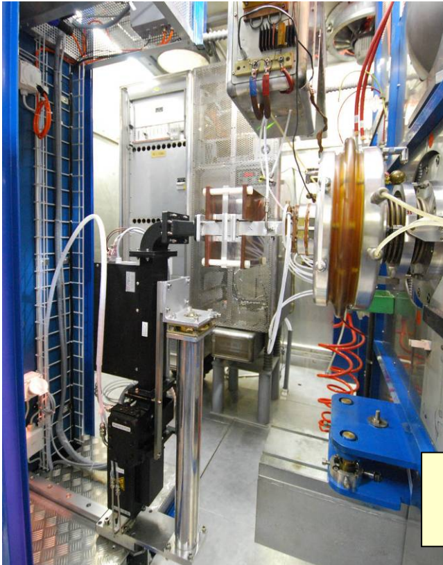
ECR source in place
