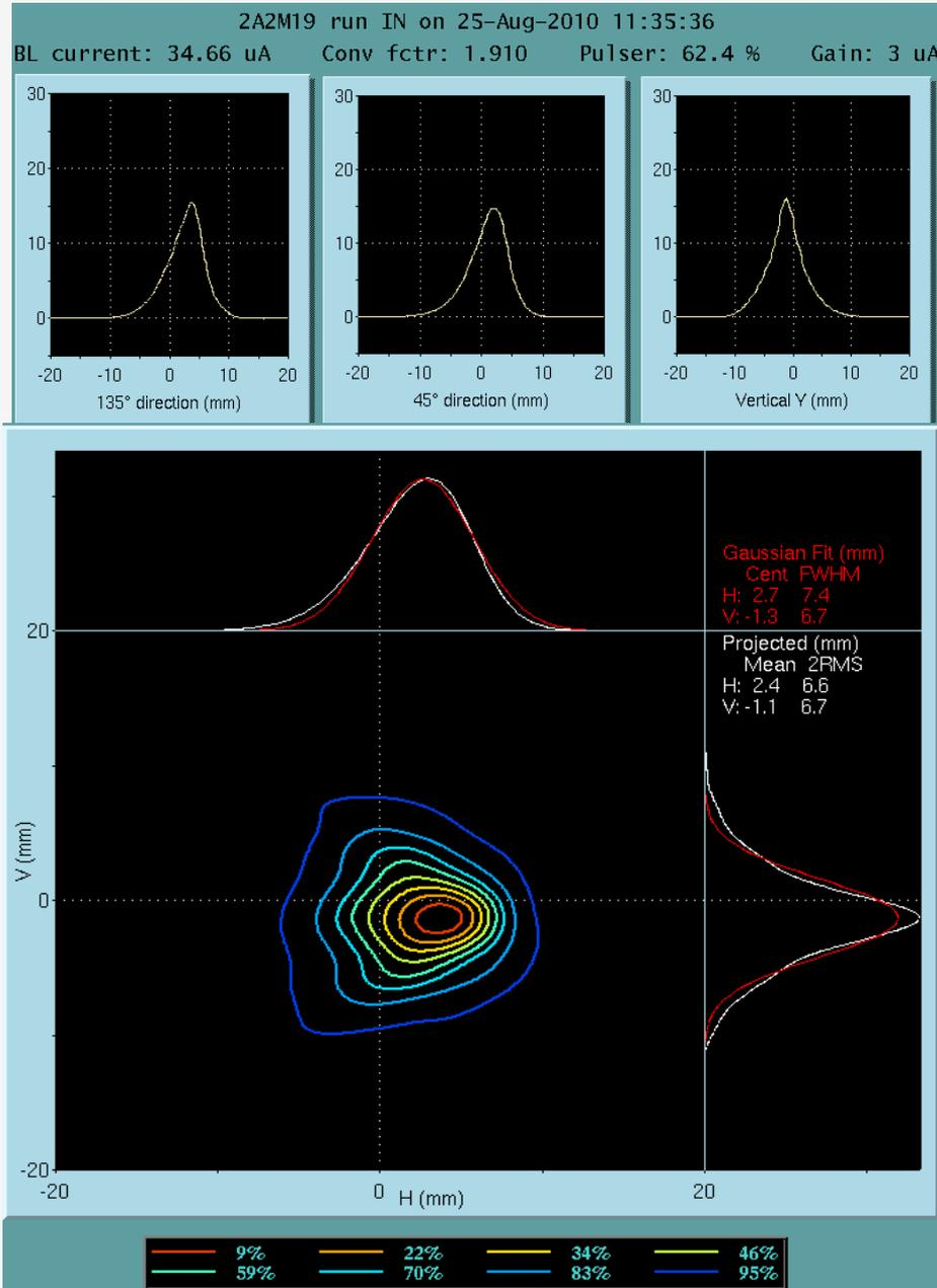
To protect the ISAC target, and to get the most out of it, it is important to monitor that the density of beam on the target remains within specifications. But it's difficult to measure, so we implement the MENT algorithm to reconstruct tomography of beam distribution on the target, by using a 3-wire monitor measured profiles in the vertical, +45° and -45° directions.
