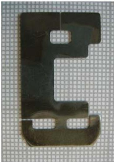
Foil thinning displaces the peak of the stripped beam charge distribution toward lower charge states. Foil thickness measured with  $\alpha$  source.
