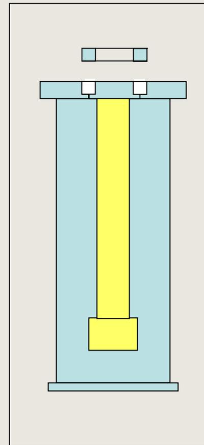
**4. Weld inner conductor to cavity and add reinforcing ring**
