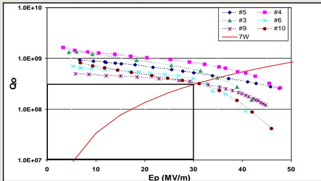
• Single cavity tests have an average performance of  $E_p=35\text{MV/m}$  at  $P_{cav}=7\text{W}$
