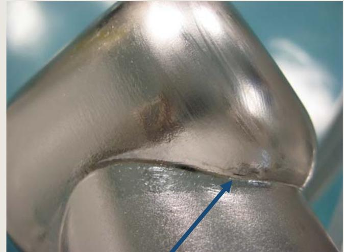
Vacuum leak appears in weld region after BCP etching
