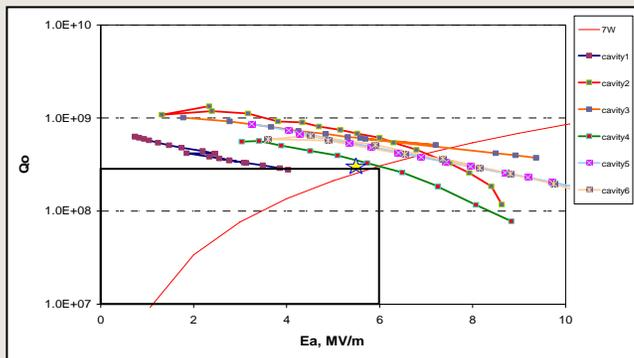
• Performance on-line with fast cooldown shows performance is recovered - one cavity shows signs of pollution; will try to recover with conditioning
