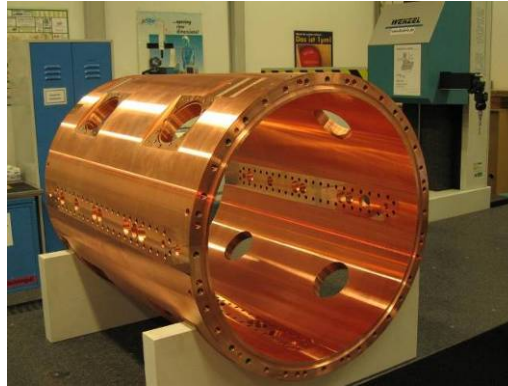
Construction of RFQ: first segment finished in a few days !
