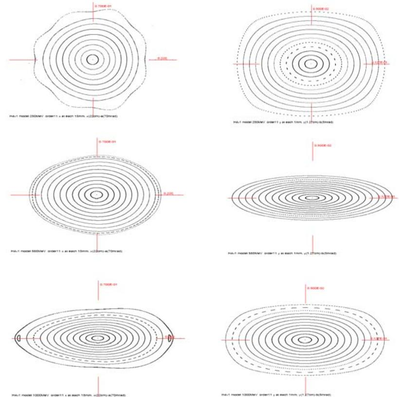
Dynamic aperture at 250, 585, and 1000 MeV – step size is 1.5 mm in the horizontal (left) and 1 mm in the vertical (right).
