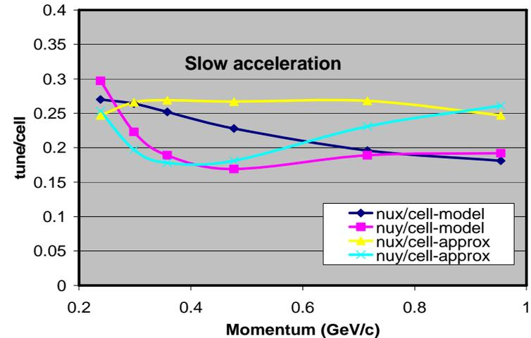
Control of tune variations in a nonscaling FFAG with a constant gradient
