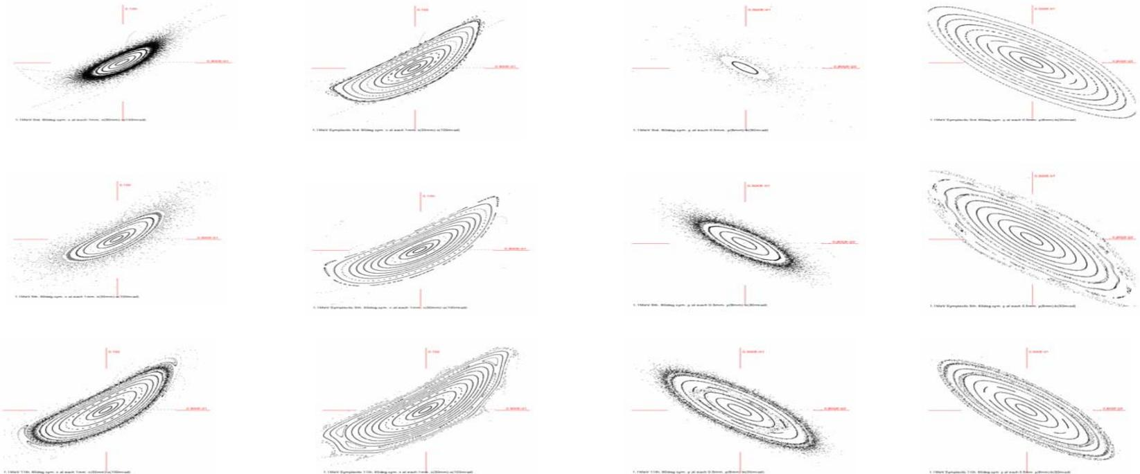
Tracking in a model non-scaling six-fold symmetric FFAG for horizontal (left pairs) and vertical (right, pairs) with 3<sup>rd</sup> (top), 5<sup>th</sup> (middle), and 11<sup>th</sup> (bottom) out of plane expansion, with focusing from an azimuthal field variation expressed as a single Fourier mode as well as edge focusing. With (left) and without (right) Expo symplectification is shown.
