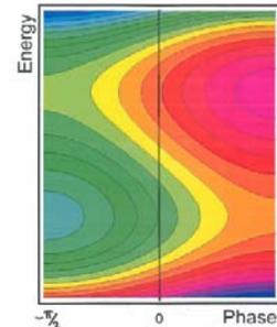
**Characteristics– tune sweep/unit cell, parabolic pathlength on momentum (small radial apertures); serpentine (rapid) acceleration – beam “phase-slips”, crossing the peak 3 times, accelerating between rf buckets**
