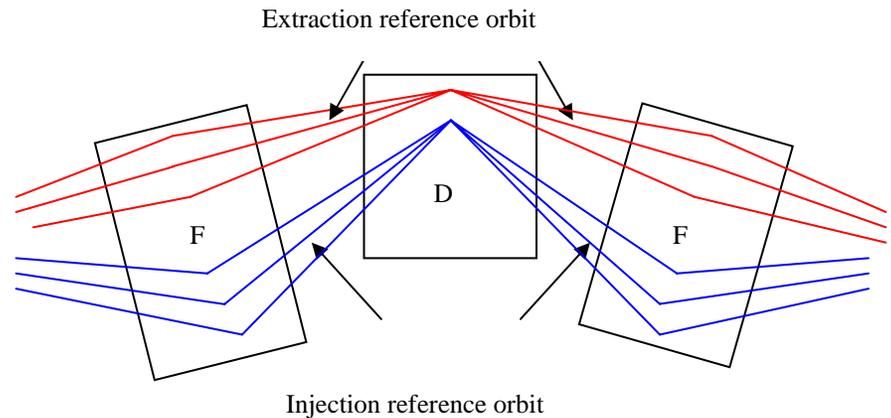
1½ cell of a nonscaling, linear-field FFAG for muon acceleration showing the compression of orbits in particular in the center magnet.
