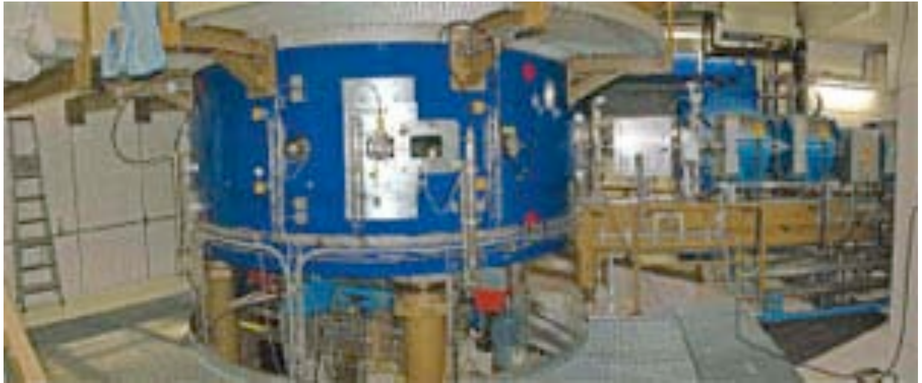
The PSI SC Accelerator. Diameter 3.25 m, 250 MeV protons Built by ACCEL (based on design by Hank Blosser)
