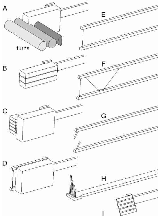
Figure 4: Schematic view of different radial probe heads.
