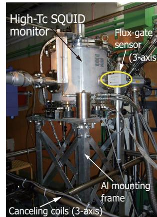
Figure 5: High-Tc SQUID monitor equipped with Al mounting frame and the noise cancellation system, which was installed in transport line between fRC and IRC.
