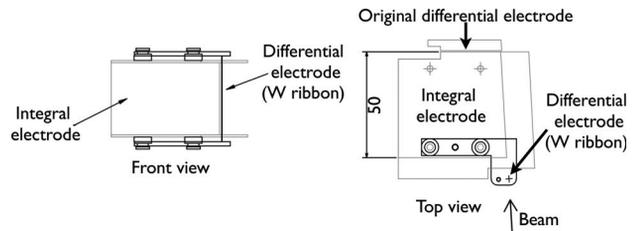
Figure 3: Modification of electrodes for SRC main radial probe. A tungsten ribbon (width : 0.3 mm) is introduced in front of the integral electrode instead of the original differential probe.
