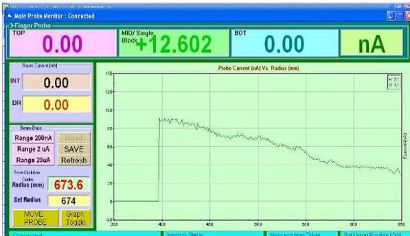
Figure 3: Current vs. radius for the  $Ne^{3+}$  beam
