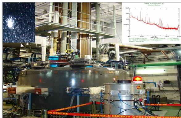
Figure 1: Superconducting cyclotron with first beam spot on left hand corner and gamma spectroscopy of the irradiated target in the right top corner
