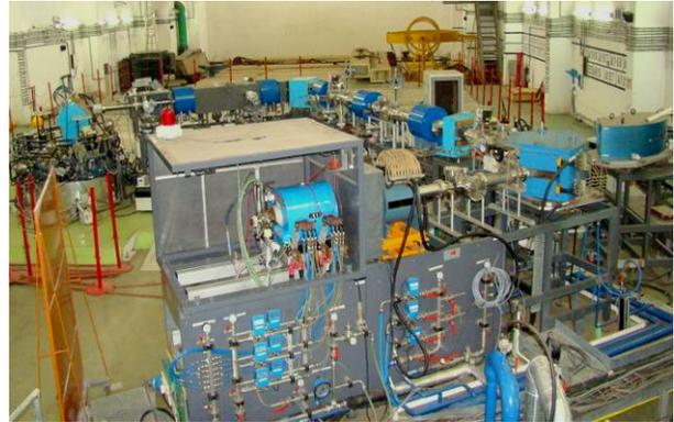
Figure 5: Installed ECR Ion Source and Injection Line
