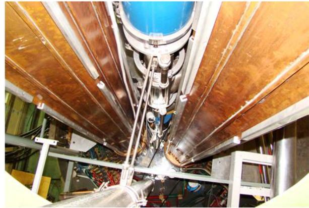
Figure 6: Vertical injection line on top of yoke
