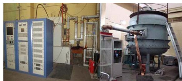
Fig. 15 High power RF cavity test stand.
