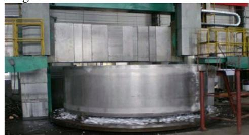
Fig. 10 The vacuum chamber in machining process.
