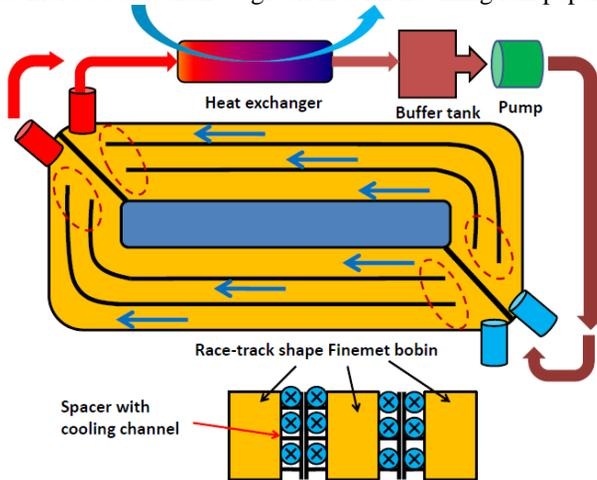
Figure 4b: Cooling system of the induction cell.
