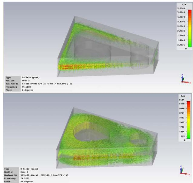
Figure 16: E-field and H-field distributions by MWS
