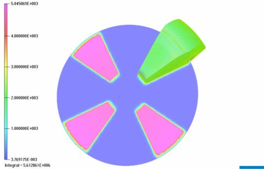
Figure 12: B-fields of simulation by TOSCA
