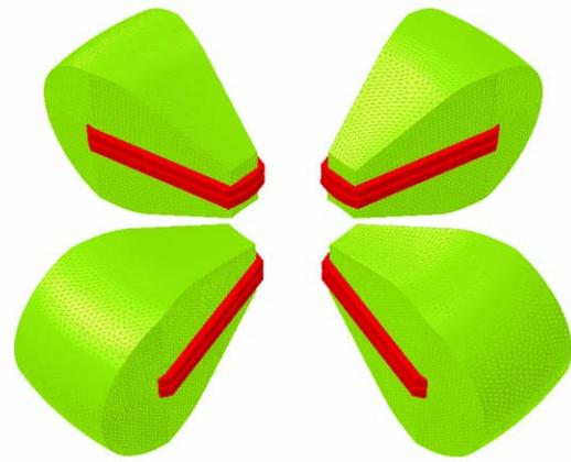
Figure 9: Meshes for magnet simulation by Opera3D
