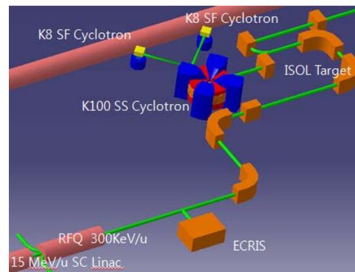
Figure 2: Layout of the cyclotron and ISOL
