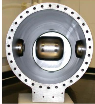
Fig. 4: Phase II cavity after etching.
