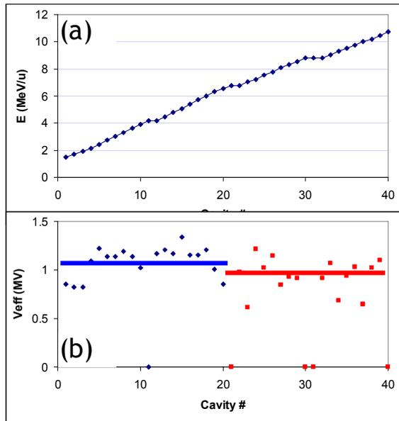
Fig. 8: Results from first acceleration of a  $^{16}\text{O}^{5+}$  beam. (a) A plot of beam energy after each cavity and (b) a plot of the effective voltage of each cavity; blue and red lines indicate the average values for Phase I and Phase II respectively.
