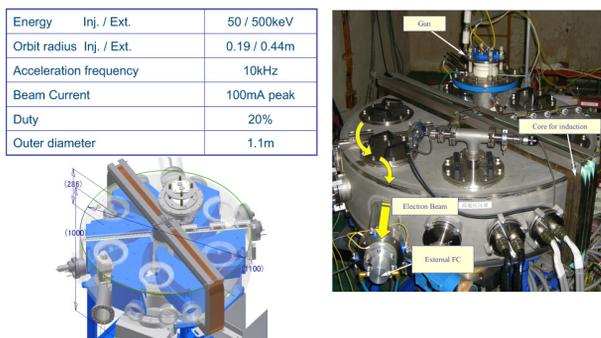
Figure 7: Electron FFAG developed at NHV Co.
