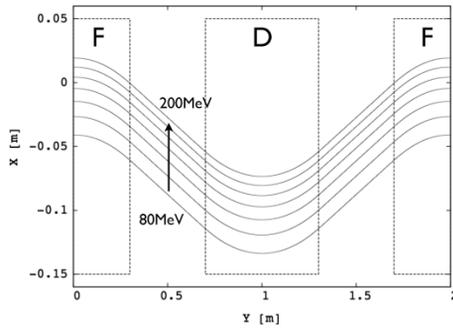
Figure 1: An example of the scaling FFAG straight line:particle is proton and energy range is 80MeV to 200MeV.
