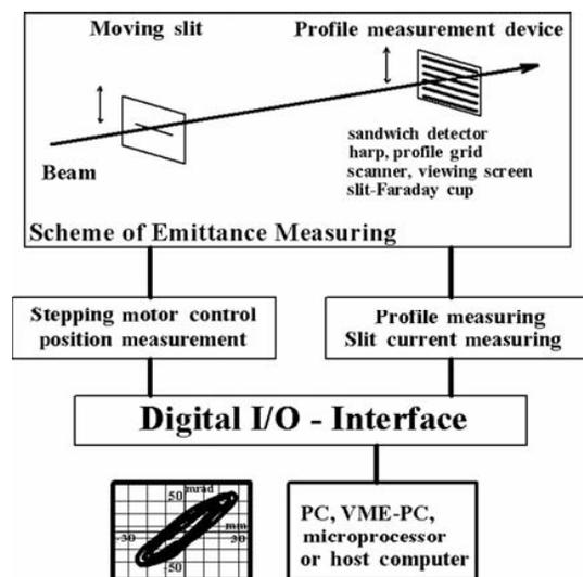
Figure 6: The scheme of measurement in slit-grid system.
