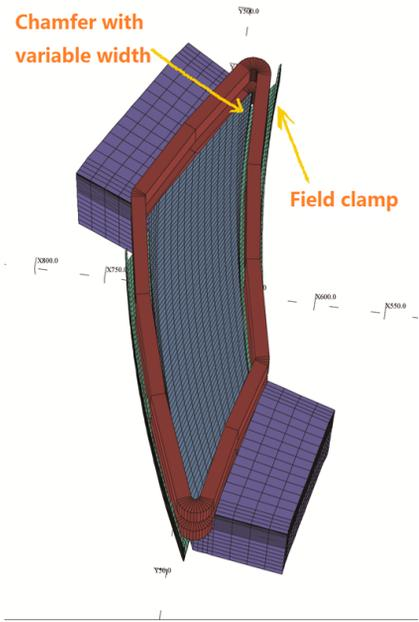
Figure 2: TOSCA magnet model with variable gap
