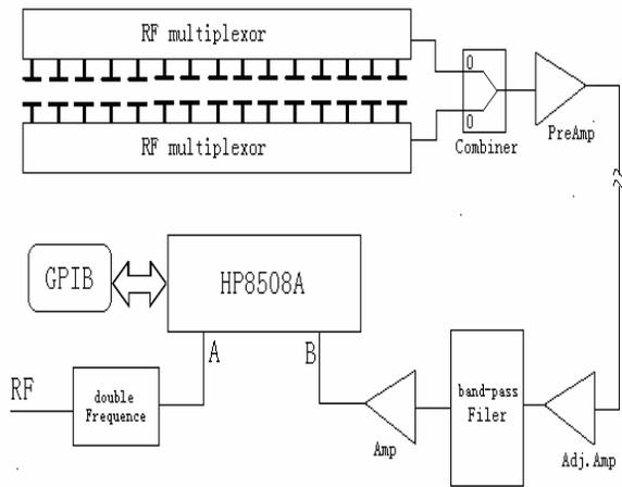
Figure 1: The diagram of beam phase measurement structure.
