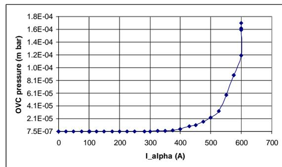
Figure 2: Vacuum reading during increase in coil current
