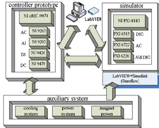
Figure 1: Hardware structure of HIL platform.
