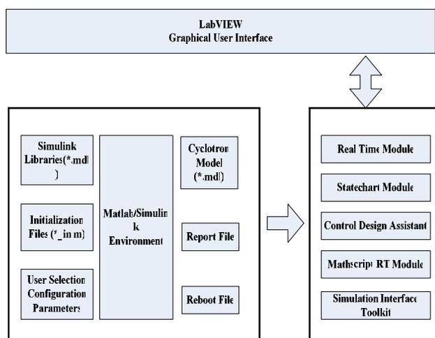
Figure 3: Software structure of HIL platform.
