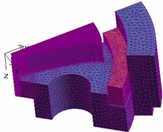
Figure 1: Model of the magnet with mesh.
