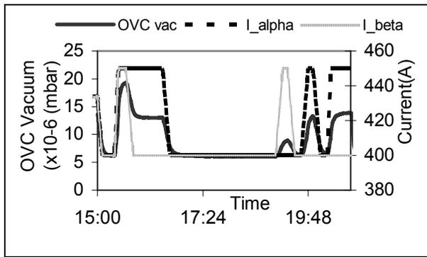
Figure 2: Variation of OVC pressure with coil current
