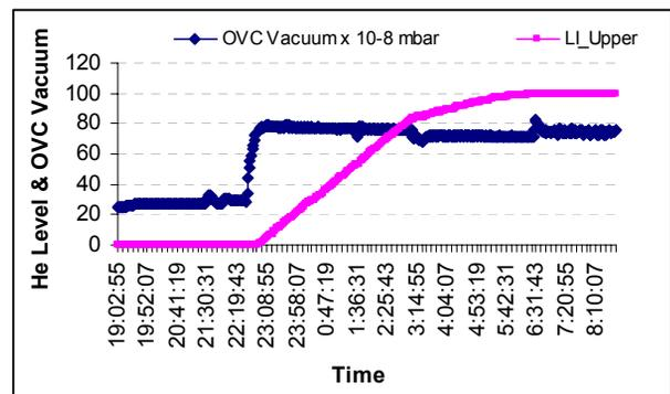
Figure 1: OVC vacuum during liquid helium filling up
