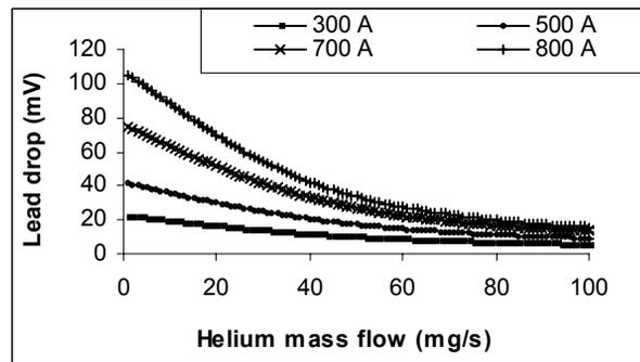
Figure 4: Simulated lead voltage drop for various excitations
