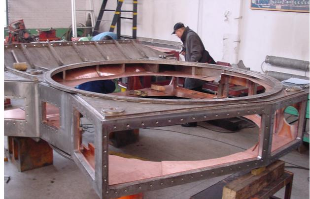
Figure 1: SFC double-deck vacuum chamber
