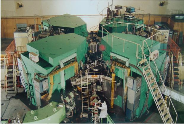
Figure 2: SSC (vacuum chamber is between the magnets)
