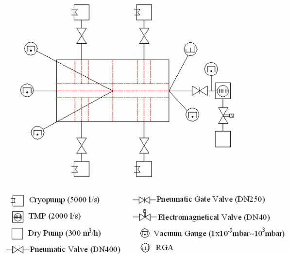
Figure 4: The vacuum equipment layout of the cyclotron
