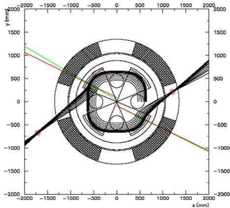
Figure 6: Equilibrium orbits and extracted trajectories for H<sup>-</sup> and protons respectively.
