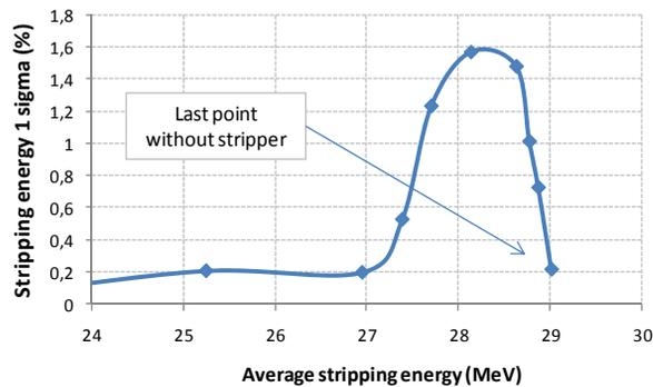
Figure 4: Effect of the 2Q<sub>r</sub>=2 resonance on the H<sup>-</sup> beam.
