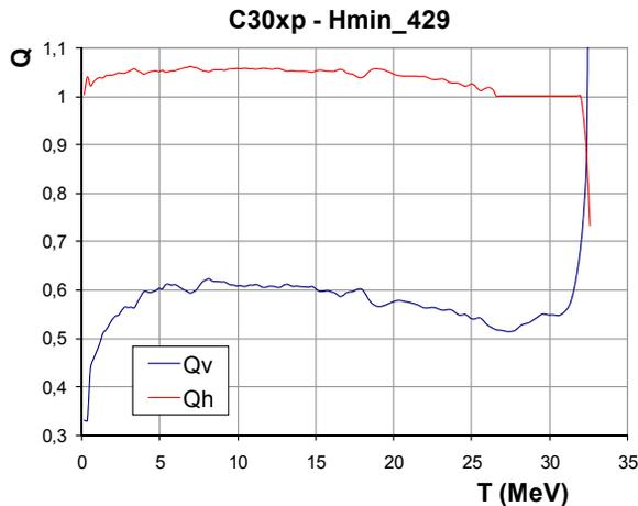
Figure 3: Locking on the 2Q<sub>r</sub>=2 resonance for H<sup>-</sup> on early Cyclone 30xp models (flat plateau on the red curve).
