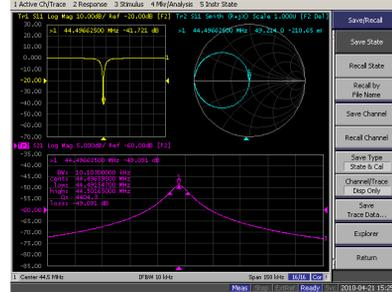
Figure 6: The loaded Q value of the cavity
