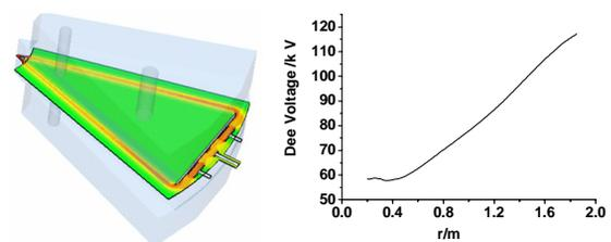
Figure 2: E-Field and the Dee voltage distribution
