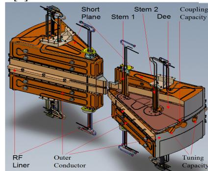
Figure 1: The structure of two stem cavity.
