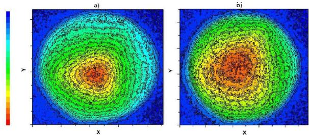
Figure 2: CCD images in false colours of an Ar plasma at the extraction region of the source. In a) the biased disk voltage is -200 V and the extracted  $Ar^{8+}$  current is 450  $\mu A$ , while in b) the disk floats at -60 V and the extracted  $Ar^{8+}$  current is only 200  $\mu A$ .
