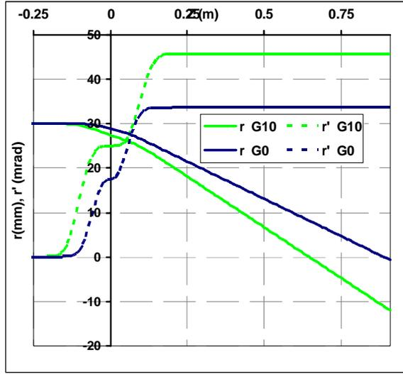
Figure 3: The distance  $r$  and angle  $r'$  of the particle are given by solid and dotted lines at different gap  $G=0$  cm and 10 cm respectively.
