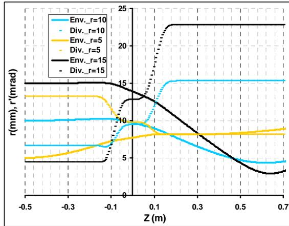
Figure 4: The beam envelopes (Env.) and divergence (Div.) with initial beam width  $2r$  and angular width  $2r'$  of the beam of phase space area taken to be  $=r r'=200$  mm-mrad passing through the MEL for  $G=5$  cm gap.
