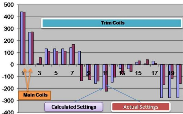
Figure 7: Comparison of the main coil & trim coil current settings
