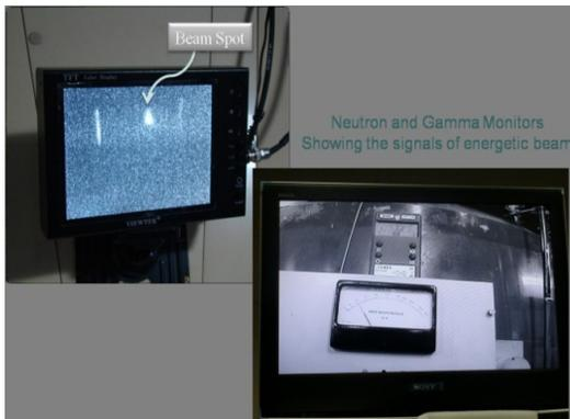
Figure 9: Beam spot on Borescope at 650 mm radius
