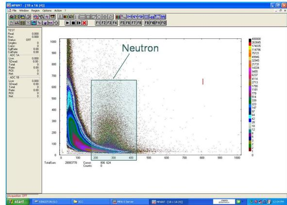
Figure 10: Neutron-Gamma discrimination with liquid scintillator.
