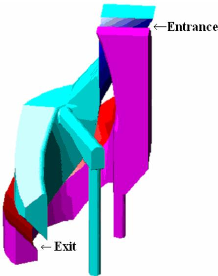
Figure 1: Optimized electrode geometry of the inflector.
