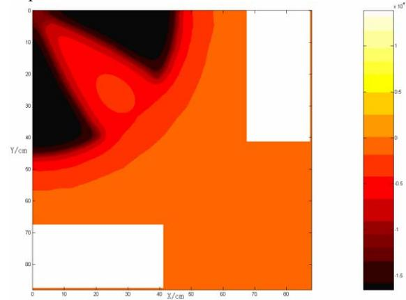
Figure 1: magnetic field map of the median plane
