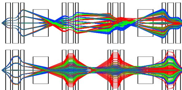
Figure 4: The element-by-element tracking result of the s-shaped pre-separator using 7<sup>th</sup> order Taylor map. Upper envelop is for horizontal plane and the lower one is for vertical plane. The maximum slope of rays is 40 mrad; the amplitude is 1 mm and the momentum deviation is 1.4%.
