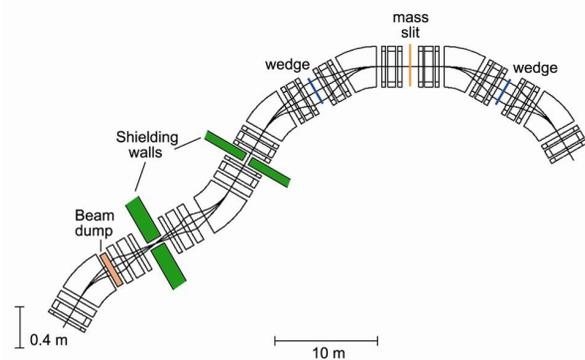
Figure 1: Configuration of a separator under consideration.
