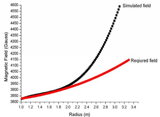
Figure 6: Simulated versus required field
