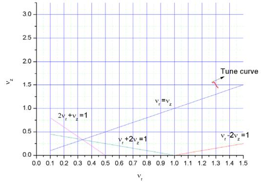
Figure 10: Tune diagram
