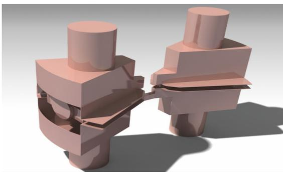
Figure 5: Cavity design using 3D CAD
