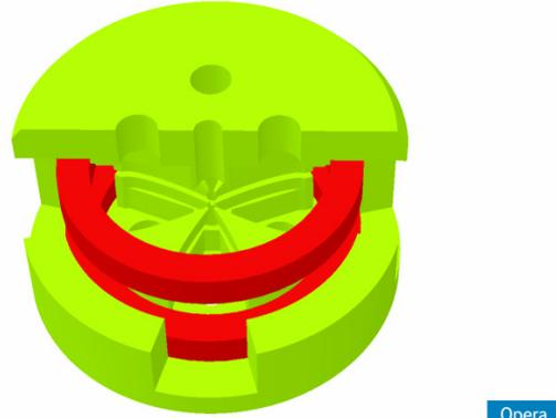
Figure 1: Model of magnet system and main coils.
