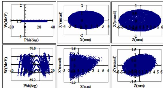
Fig.4 The phase space distributions of initial beam (upper), extracted 70MeV H<sup>+</sup> beam on the stripping foil.
