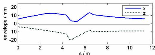
Fig. 6 Total beam envelopes along one beam line.
