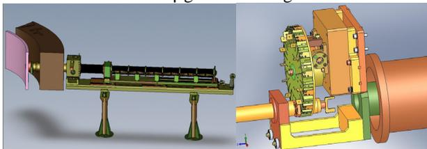
Fig. 2 Stripping Extractor and Foil changing devices.
