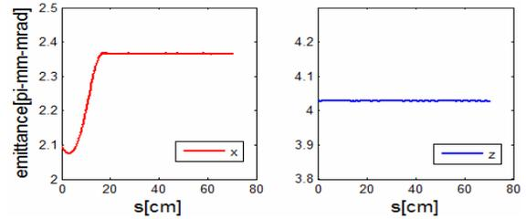
Fig.3 Emittance of the extracted beam
