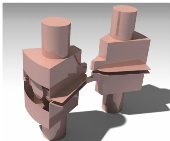
Figure 6: Final RF cavity design using CATIA V5
