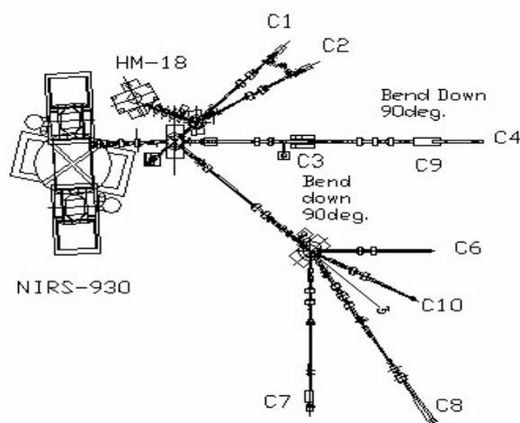
Figure 1: Layout of cyclotrons and beam lines.
