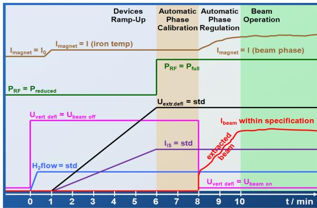
Figure 1: Timing diagram of the transition “RF ready” to “Beam ready”.
