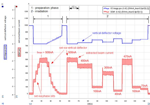
Figure 4: Sequence of the beam current setting procedure.
