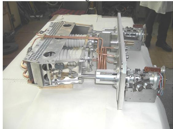
Figure 6. Electrostatic deflector
