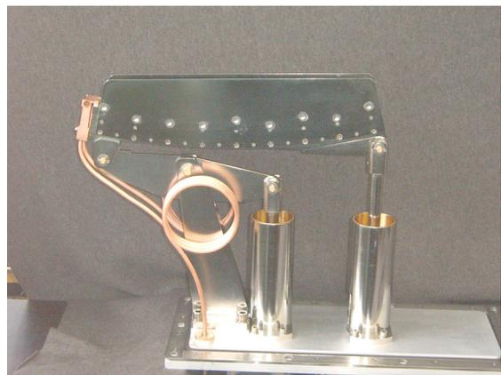
Figure 7 Magnetic channel
