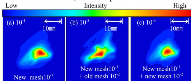
Figure 2: Comparison of beam intensity profiles on the target with a previous short interval of meshes: (a) standard for comparison with only a new mesh of opening ratio of  $10^{-1}$ , (b) added an old mesh of opening ratio of  $10^{-2}$  ( $\phi$  0.1 mm), (c) added a new mesh of opening ratio of  $10^{-2}$  ( $\phi$  0.01 mm). These profiles were obtained from the optical density of irradiated radiochromic films, GAFCHROMIC films (HD-810, International Specialty Products) [3].
