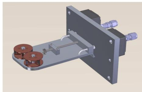
Figure 6: Extraction probe
