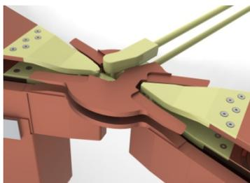
Figure 3: Internal ion source
