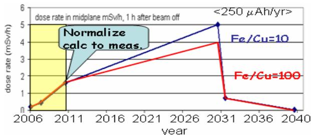
Figure 7: Estimated dose rate in the mid plane between open pole caps, based on the 2010 measurements and scaled calculated dose rates, assuming 250  $\mu\text{Ah/y}$ .
