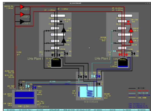
Figure 3: GUI of liquid helium system overview
