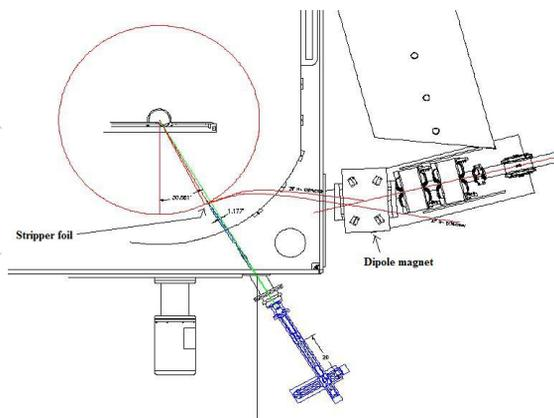
Figure 5: Extraction for H<sup>-</sup> and D<sup>-</sup> beams.
