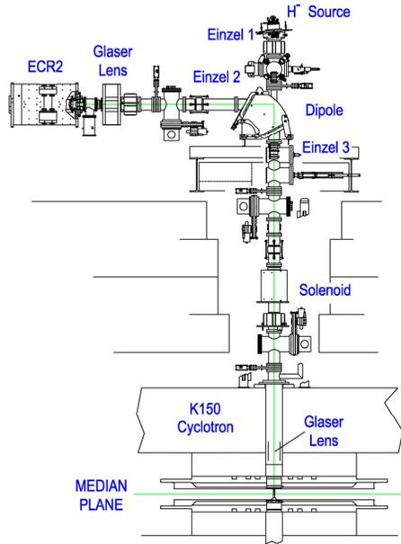
Figure 2: Injection line for the K150.
