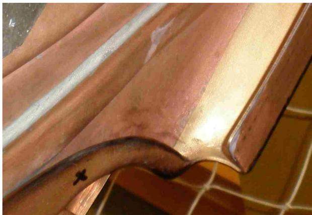
Figure 2: Detail of the gold coated outer perimeter of the acceleration electrodes.
