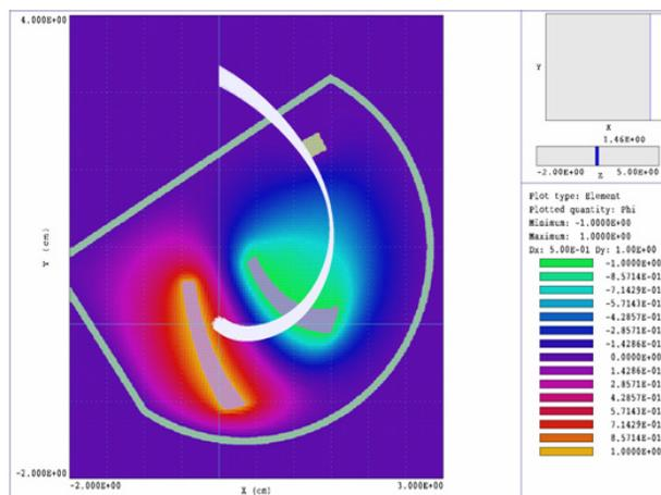
Figure 3. Field map solutions (top view) and 25 kV  $\text{Ar}^{9+}$  trajectories starting at  $x=0$  cm,  $y=0$  cm travelling in the negative  $z$ -direction. The initial beam diameter is 2 mm. The applied voltages to the top and bottom electrodes are -7.75 and 7.75 kV respectively.
