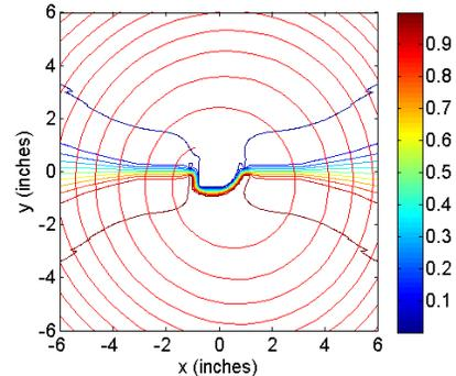
Figure 6. The first few turns of a 25 kV  $Ar^{9+}$  ion beam in the new center region of the 88-Inch Cyclotron and equipotential contours of the electric field. Colorbar indicates fraction of Dee voltage.
