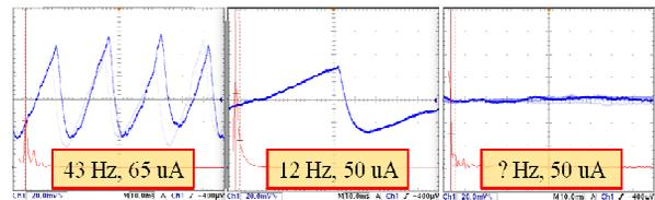
Figure 3: A beam of  $^{40}\text{Ar}^{7+}$  at a 24.43 kV extraction potential is shown on an FFT oscilloscope for microwave powers of 305, 310, and 315 W. The AC coupled signal is shown as the upper trace in blue, with the AC component of the DC signal being 2.7%, 1.9%, and  $< 0.1\%$ , respectively.
